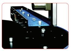
A soft non-slip sprocket driven conveyor safely handles the parts onto the rotary table.
